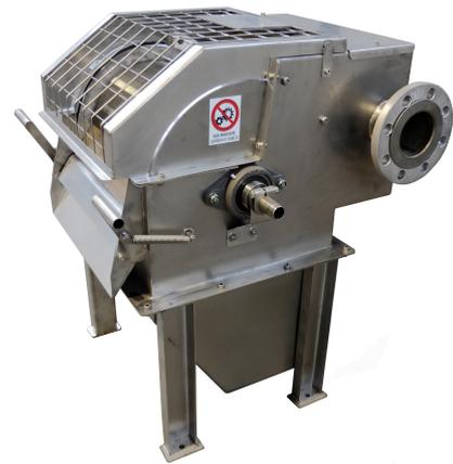
**MP SCREEN** is connected to a back washing system inside the cylinder, to be activated intermittently in the case of wastewater with particularly difficult and clogging properties.
